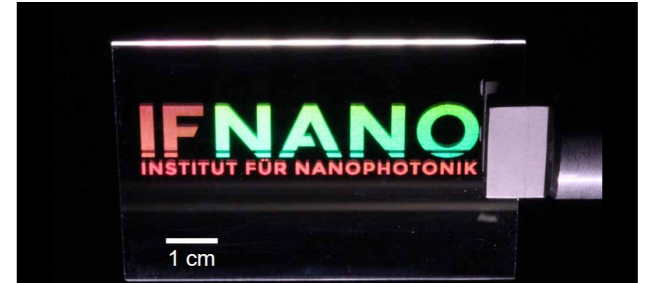
Figure 2: Diffractive mark on glass made by phase mask projection. The area appearing red has a structure period of 2 \mu\text{m} , the area looking green a period of 3 \mu\text{m} .
